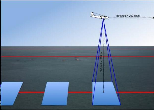
Fig. 1: Marine environment marine survey using airborne photography system (images of 400m x 300m)
