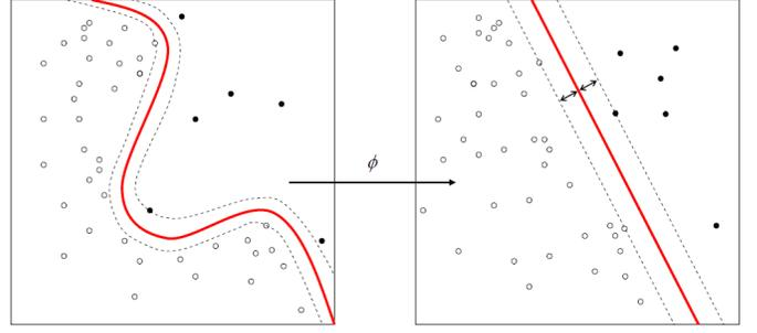
Fig. 4: Trick of non-linear transformation  $\Phi(x)$  in SVM (Support Vector Machine)
